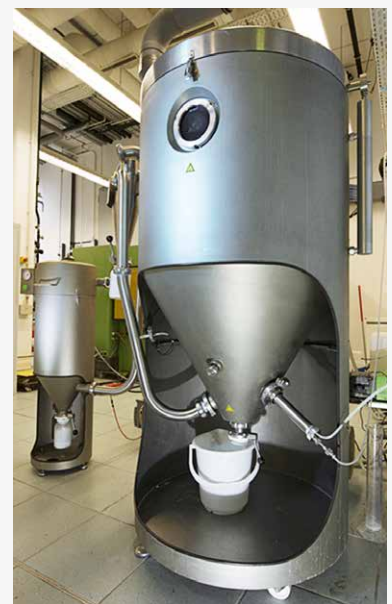
Scale-up equipment with 100 L batch reactor (left), semi-continuous centrifuge (center) and a pilot-scale spray dryer (right).
