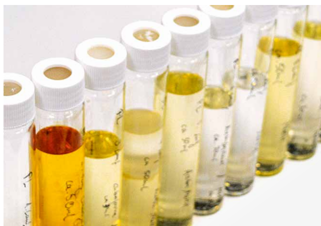
Figure 3 Phase separation of latex components (left) and their composition in dandelion rubber (right).
