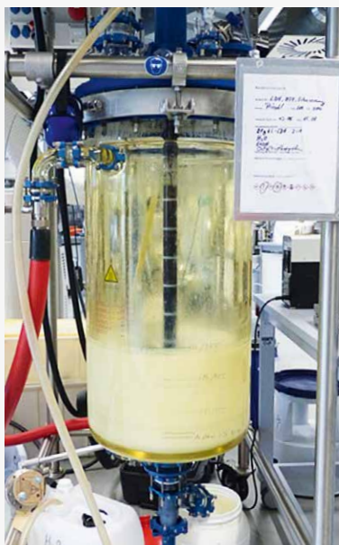
Scale-up equipment with 100 L batch reactor (left), semi-continuous centrifuge (center) and a pilot-scale spray dryer (right).
