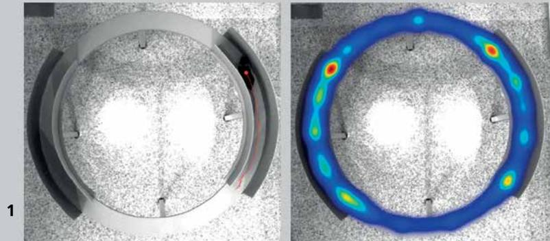
1 *Elevated plus maze test for measuring anxiety using Noldus EthoVision*
