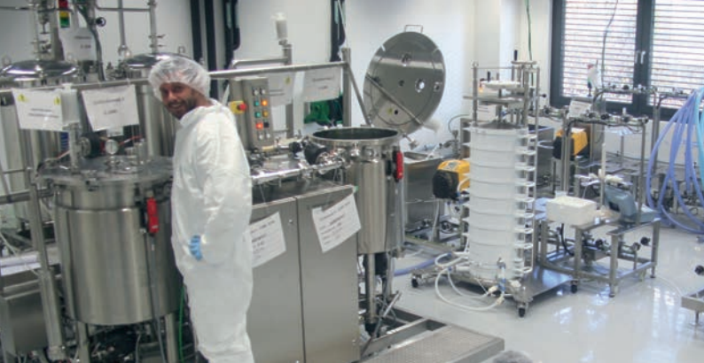
800 L extraction and filtration plant in monitored environment
