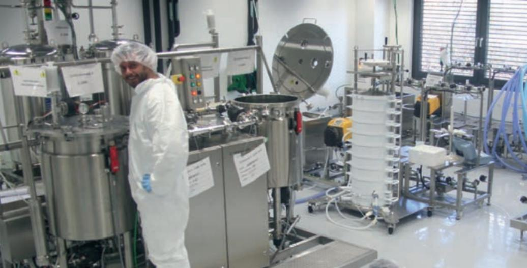
800 L extraction and filtration plant in monitored environment
