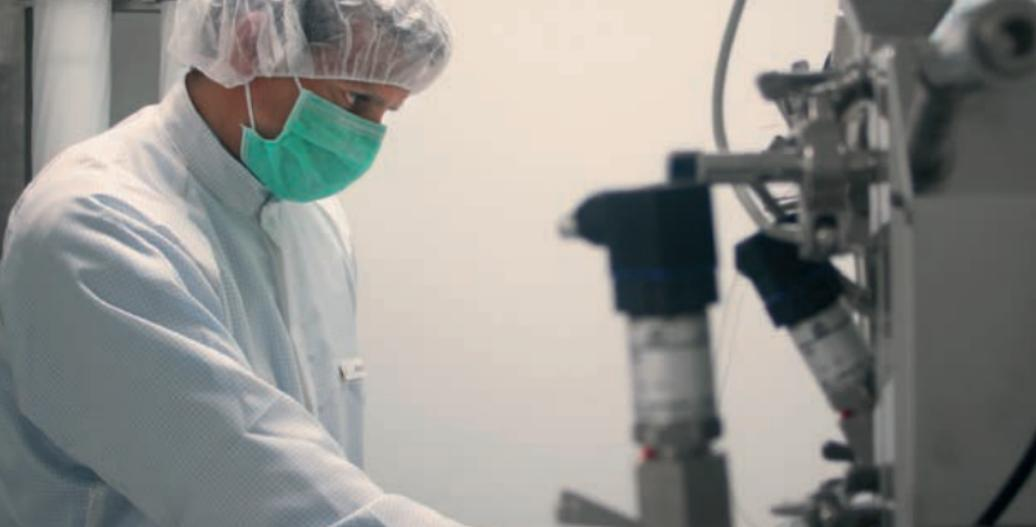
Diafiltration during downstream-processing of a drug substance
