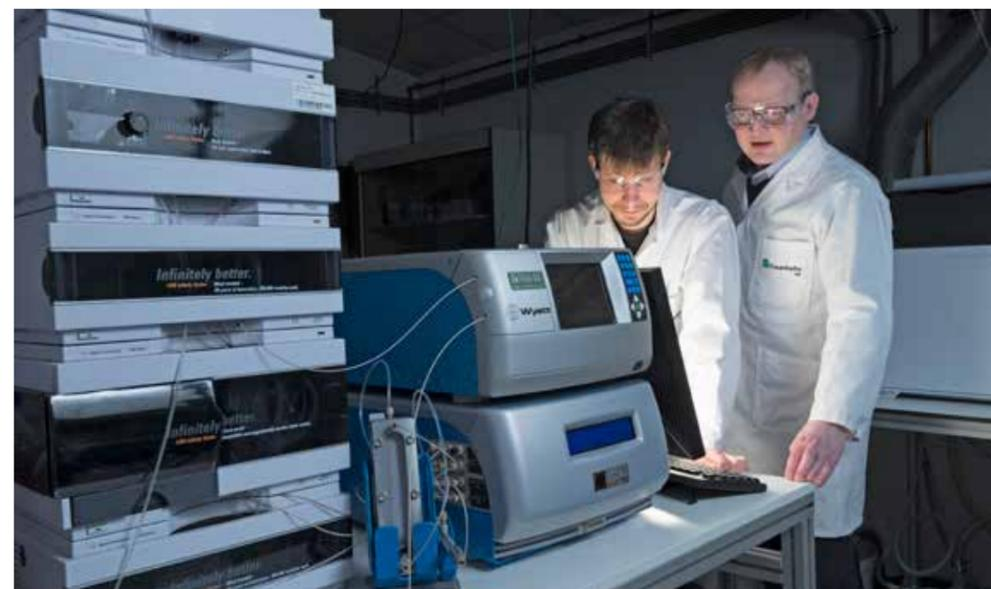
Boris Meisterjahn and Prof. Dr. Christian Schlechtriem in the laboratory with the AF4 system (used to fractionate nanoparticles). Fraunhofer IME offers state-of-the-art techniques for the characterization of nanomaterials.
