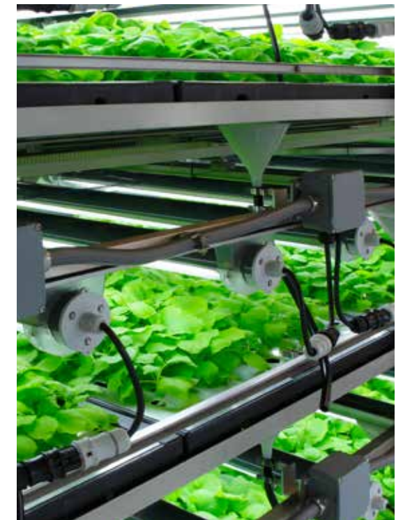
Using an automated system, the seeded trays are placed in stainless steel growth racks in a strictly climate controlled room. The plants are grown for 4-5 weeks until they are mature enough to undergo vacuum infiltration.
