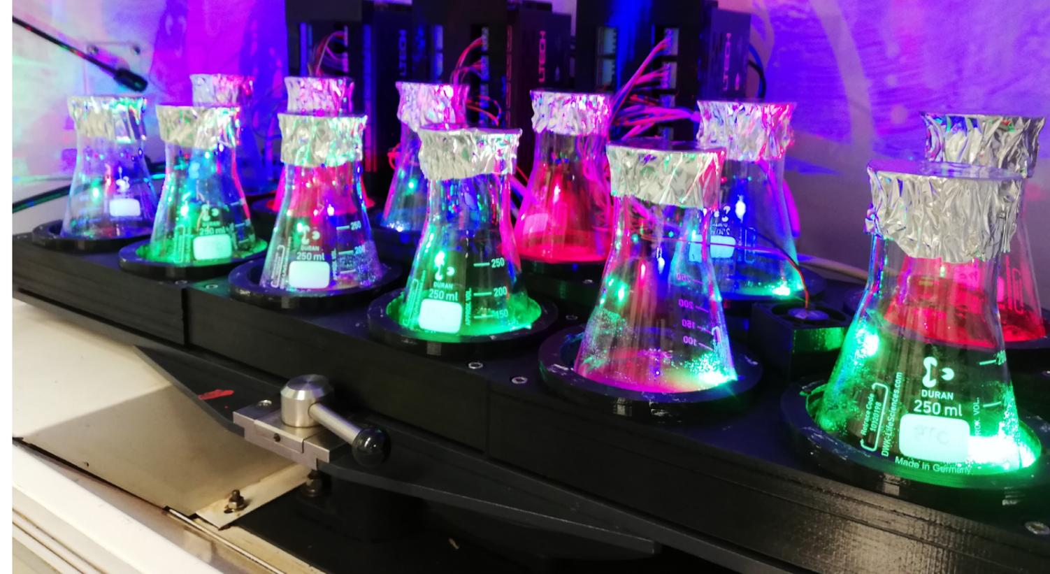
The LEDitSHAKE system: 12 individually lit conical flasks in a shaking incubator.
