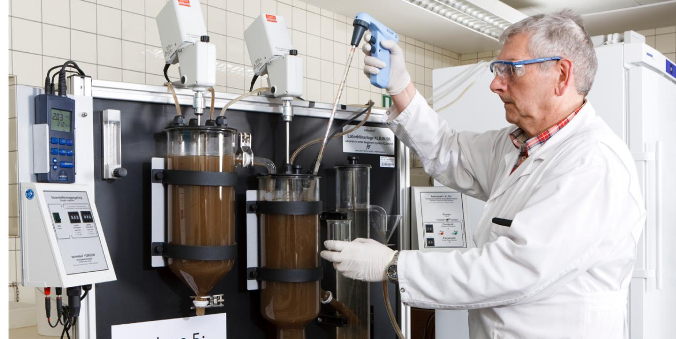
*Behavior of Ag nanoparticles in the sewage plant and adsorption to sewage sludge.*
