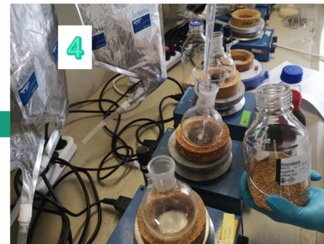
4 Addition of chloroform and NaOH
