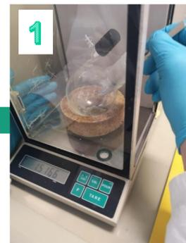
1 Weighing of 1.5 g sample into Schlenk flask
