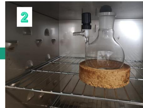
2 Drying at 105 °C for 30 min
