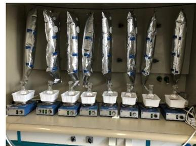
Figure 1: Experimental silylation set-up
