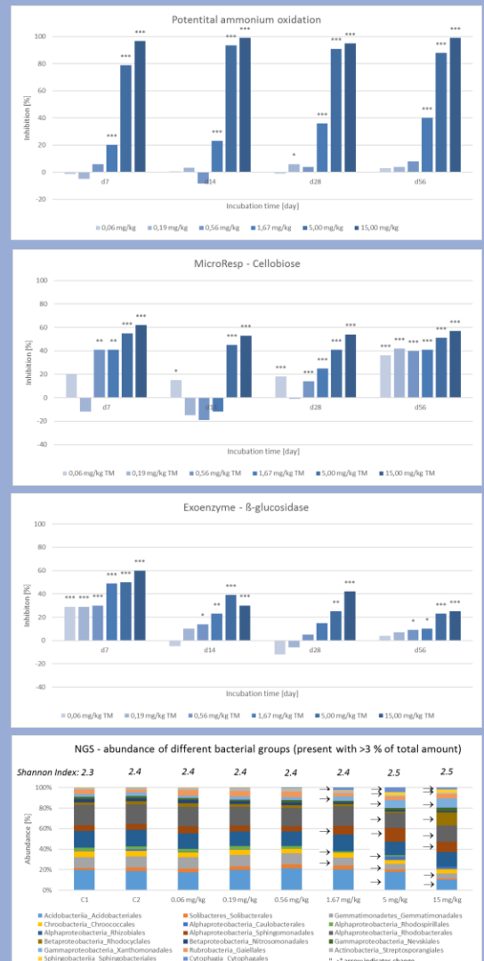
Figure 1: Effect of a silver nanomaterial on the soil microflora - examples for results determined with the four approaches.
