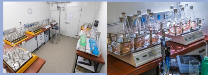
Fig. 1: Transformation / Dissolution test setup
