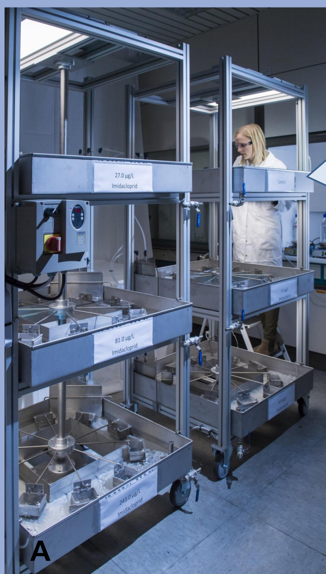
Fig 2: (A) Test system with six treatments. (B) Test container with ten circulating replicates. (C) & (D) Test vessel with stonefly larva.
