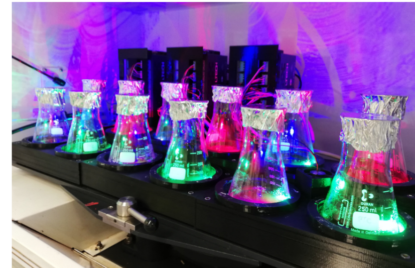
LEDitSHAKE lighting system to optimize plant cell cultures for secondary metabolite production.
