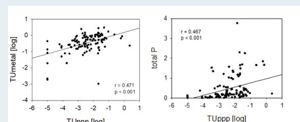
**B) Spearman rank correlation** between pesticide pressure (TU<sub>ppp</sub>) and metal concentration (left) respectively total phosphorus concentration (right). TU = Toxic Unit = measured concentration / EC50, max. TU was used here
