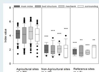
**A) Box plots** of main parameters of hydro-morphological mapping. Low index values indicate good status (Student's t-test, \*\*\*:  $p < 0.001$ , \*\*:  $p < 0.01$ )
