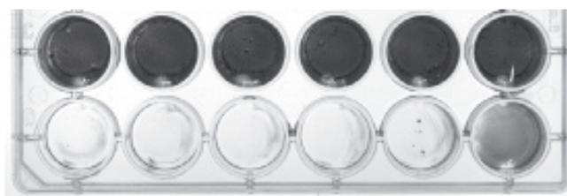
Figure 1: Assay for biofilm degradation using a microtiter plate format. Dark wells indicate functional biofilms, translucent wells degraded biofilms.
