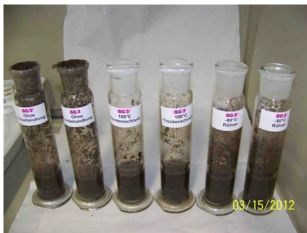
Figure 13: manure samples after autoclaving at 121 °C and different pre-treatment
