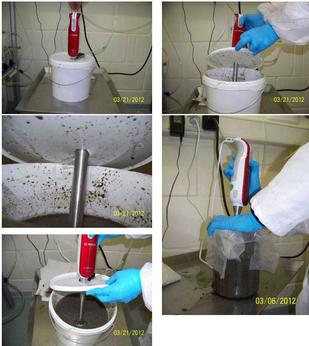
Figure 9: manure homogenization procedure while keeping anaerobic conditions
