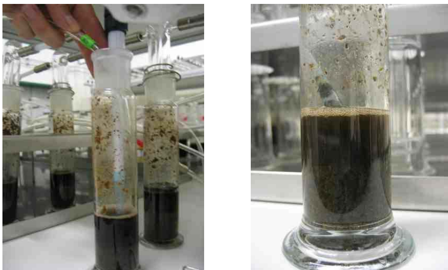
Figure 14: application under anaerobic conditions, stirring with the pipette tip, which remains in the sample
