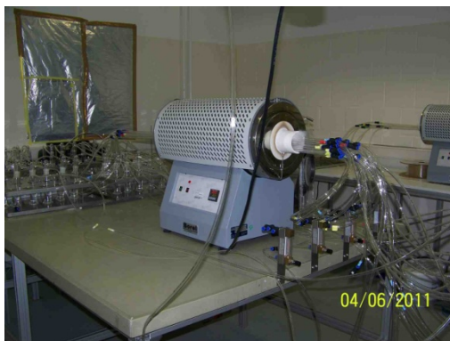
Figure 11: tube furnaces for combustion of methane to carbon dioxide and subsequent trapping in NaOH-solution
