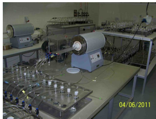
Figure 11: tube furnaces for combustion of methane to carbon dioxide and subsequent trapping in NaOH-solution
